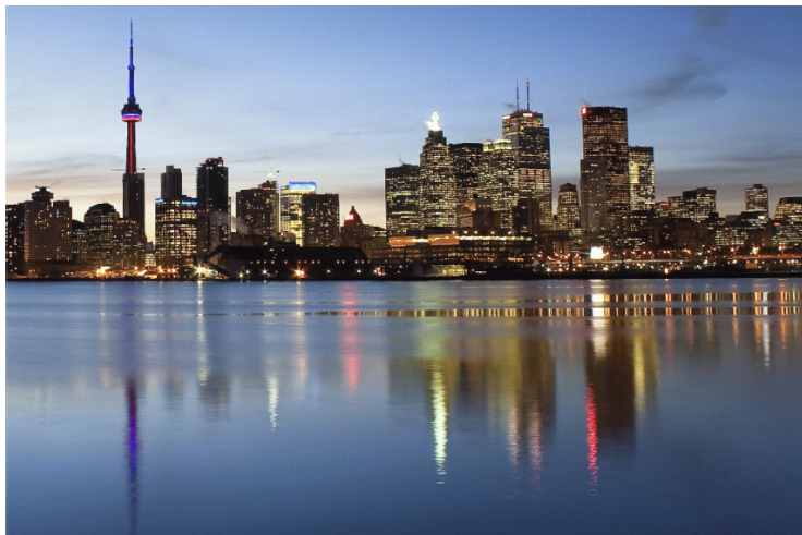
Figure 1. Reflection of lights on surface waves. At grazing angle, each wave crest results in an apparent image, causing a linear streak of images centred on the unperturbed image location. For example, the red light streak would consist of a single image at its centre in the absence of waves. The inclined sheet model for pulsar scintillation is analogous, with reflection replaced by refraction. Image copyright Kaitlyn McLachlan, licensed through shutterstock.com image ID 45186139.
