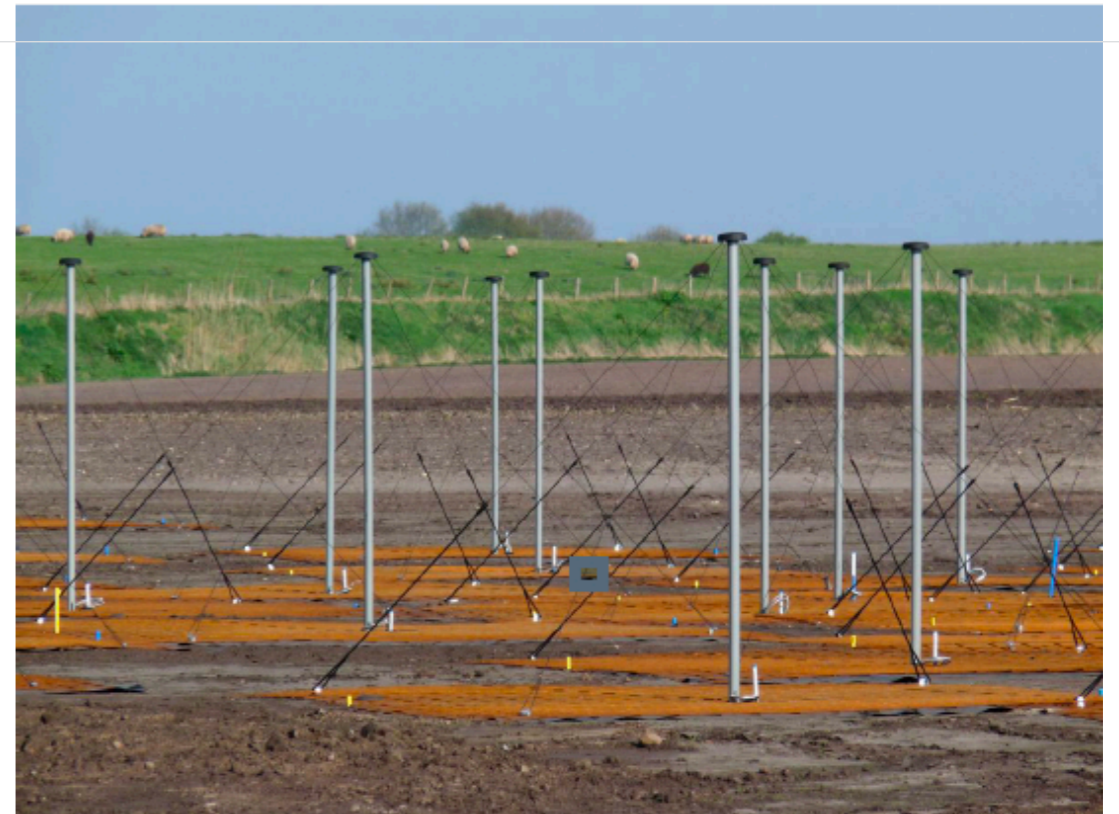
Low band antenna (LBA; 1090MHz)
