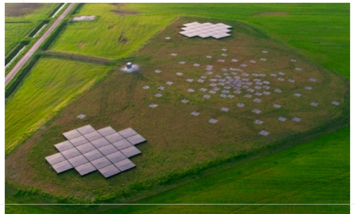
A LOFAR core station with two HBA and one LBA.
