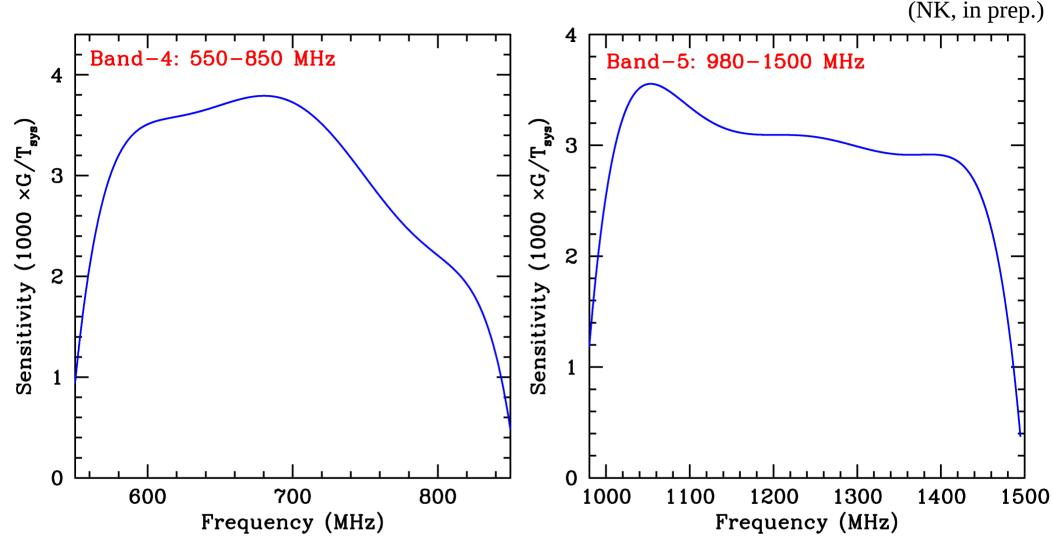
• "Band–4": 550 – 850 MHz. Remarkably clean band! Cut-off at ~ 850 MHz, to avoid cellular transmissions.
