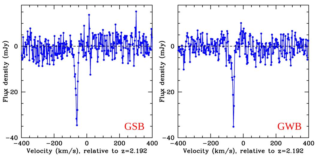
• RFI spikes replaced by noise before correlation in the GWB data. No RFI mitigation in the *simultaneous* GSB data (daytime run).
